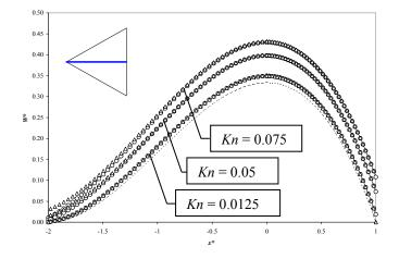
Figure 3: Equilateral triangular section - dimensionless velocity along the symmetry axis  $(y^* = 0)$ ; comparison between no slip (--), slip flow analytical results (--), MW (O) and LPBS ( $\Delta$ ) S/6 simulations for different Kn
