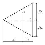
Figure 1: Equilateral triangular section.
