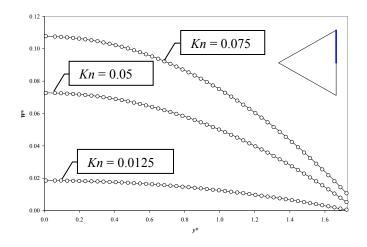
Figure 4: Equilateral triangular section - dimensionless velocity at the wall  $(x^* = I)$ ; comparison between analytical solutions (—) and MW (O) S/6 simulations for different Kn.
