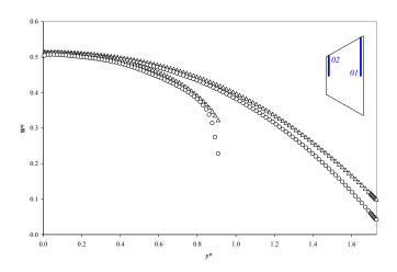
Figure 9: Trapezoidal section, dimensionless velocity at cells center near the walls ( $x^* = 0$ ,  $x^* = 1.15$ ); comparison between MW (O) and LPBS ( $\Delta$ ) simulations for Kn' = 0.0866
