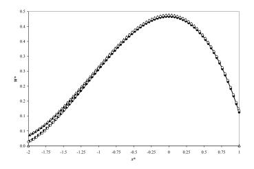
Figure 6: Equilateral triangular section - dimensionless velocity along the symmetry axis ( $y^* = 0$ ): comparison between analytical results (—), S/6 MW ( $\circ$ ), S/6 LPBS ( $\Delta$ ), S/2 MW ( $\bullet$ ), S/2 LPBS( $\Delta$ ) simulations for Kn = 0.075.
