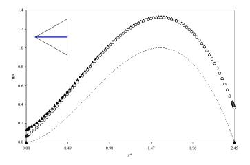
Figure 8: Isosceles triangular section, dimensionless velocity along the symmetry axis ( $y^* = 0$ ); comparison between no slip (--), MW (O) and LPBS ( $\Delta$ ) simulations for Kn' = 0.0866
