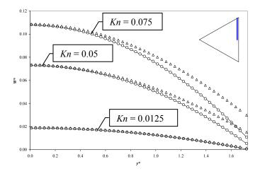
Figure 5: Equilateral triangular section - dimensionless velocity at cells center near the wall  $(x^* \approx 1)$ ; comparison between analytical solutions (—), MW (O) and LPBS ( $\Delta$ ) S/6 simulations for different Kn
