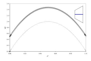
Figure 10: Trapezoidal section, dimensionless velocity along the symmetry axis ( $y^* = 0$ ); comparison between no slip (--), MW (O) and LPBS ( $\Delta$ ) simulations for Kn' = 0.0866
