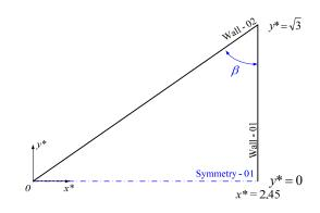
Figure 7a: Isosceles triangular section with  $D_h^* = 1.773$
