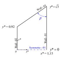
Figure 7b: trapezoidal section with  $D_h^* = 1.502$ ;  $\beta = 54.74^\circ$
