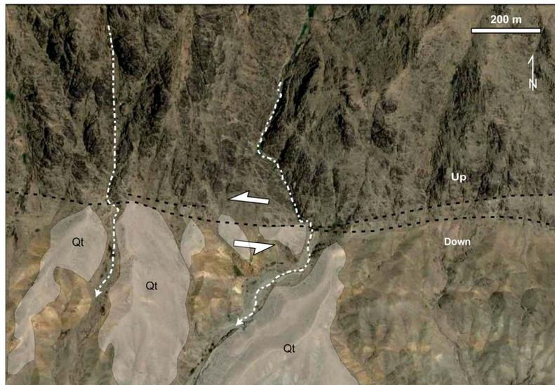
**Figure 15.** The central part of the N-dipping oblique slip fault at the Siah-Kuh Mountain front in the north of the CFZ. The fault offsets (reverse left-lateral) both Quaternary deposits and south running streams. See Figure 12a for the location.
