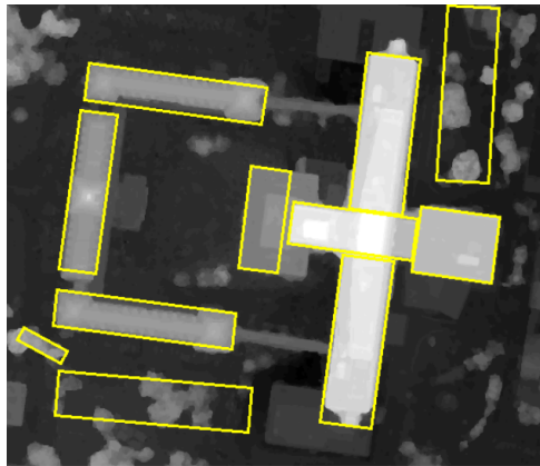
Fig. 15. Result obtained with a 20 cm aerial DEM ©IGN 2009. See also table 2. image size. However, such a large area contains enough buildings to provide a relevant idea of what we could expect while processing a whole city. In our test, we used a 50 cm GSD aerial DEM (2000×2000 pixels) on a dense urban area with almost 1100 objects. The result was obtained in about 50 minutes.
