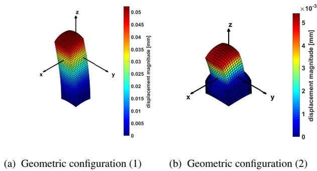
Fig. 16: Displacement amplitude under bending-traction load case
