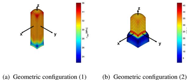
Fig. 17: Von Mises stress under pure traction load case
