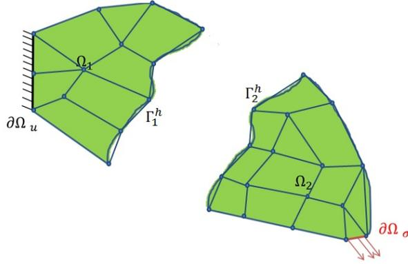
Fig. 3: Consistent discretization of the partitioned domain
