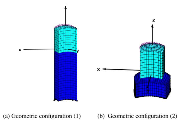
Fig. 14: Geometric configurations (1) and (2), bending-traction traction load case
