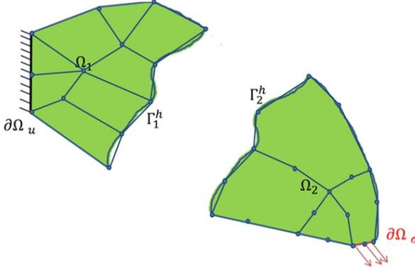
Fig. 7: Inconsistent mesh partition that introduces geometric inconsistency:  $\Gamma_1^h \neq \Gamma_2^h$ , third case different shape functions
