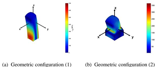
Fig. 18: Von Mises stress under bending-traction load case
