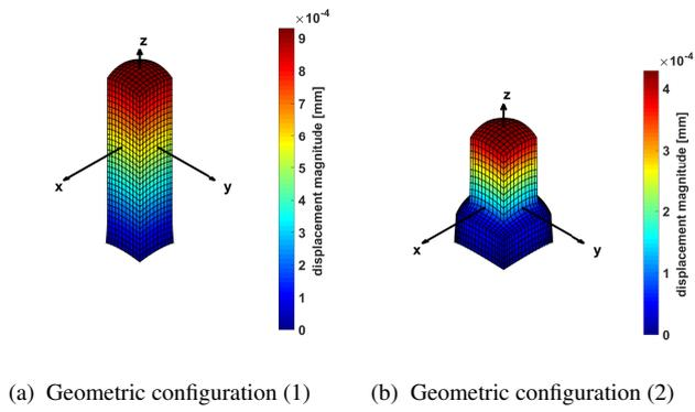
Fig. 15: Displacement amplitude under pure traction load case
