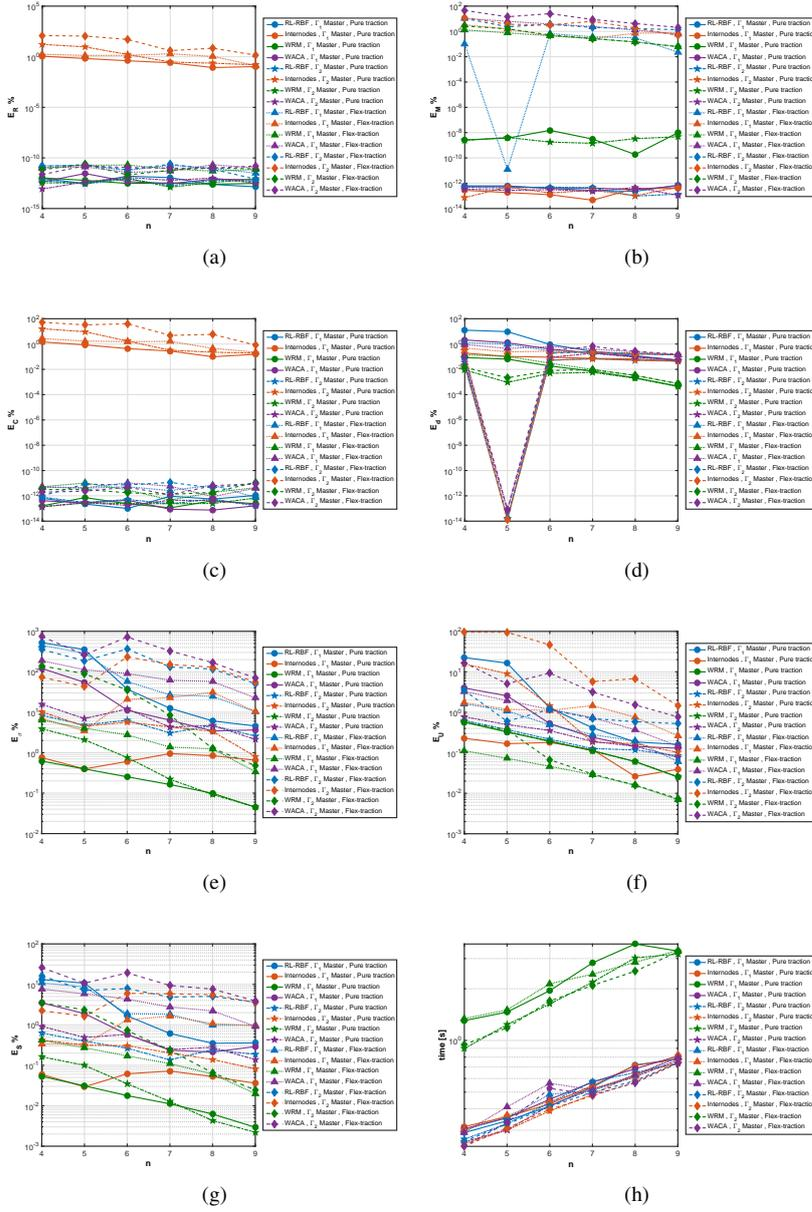
Fig. 26: Benchmark results in configuration (1) impact of  $n$  over: (a)  $E_R$ , the Resultant Force relative error, (b)  $E_M$ , the moment relative error, (c)  $E_C$ , the interface compliance relative error, (d)  $E_d$ , the displacement discontinuity relative error, (e)  $E_\sigma$ , the maximum of Von Mises stress relative error, (f)  $E_U$ , interface displacement field relative error, (g)  $E_S$ , average Von Mises stress relative error, (h) CPU time (s).
