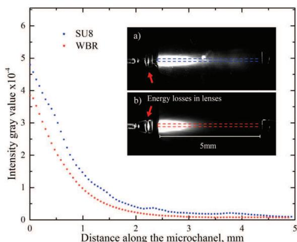
**Fig. 4.** Fluorescence images of the collimated light beam in an optical path comprising a PhLoC microfluidic channel filled with fluorescein saturated solution, excited with a 365 nm laser. a) PhLoC structure manufactured with SU-8 technology; b) PhLoC structure manufactured with low-cost DuPont dry film technology. (For interpretation of the references to color in this figure legend, the reader is referred to the web version of this article).
