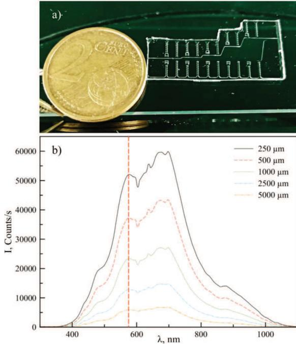
**Fig. 1.** a) Picture of a PDMS photonic lab on a chip describing 5 different optical paths (0.25, 0.5, 1, 2.5 and 5 mm) for light interrogation; b) typical intensity spectra collected through each PhLoC optical path. Vertical red-dotted line represents the wavelength chosen for PhLoCs benchmarking. (For interpretation of the references to color in this figure legend, the reader is referred to the web version of this article).
