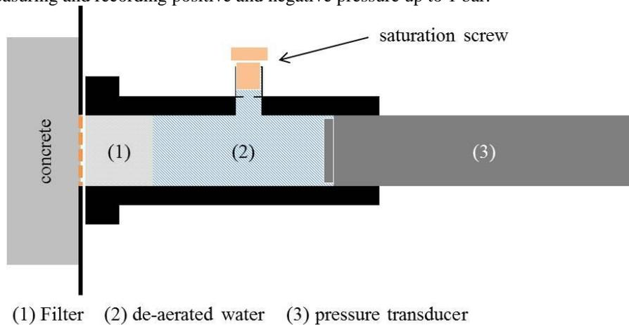
**Fig. 6.** Pore water pressure measurement system
