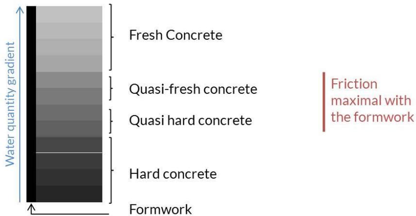
**Fig. 2.** Concrete evolution inside a slipform formwork
