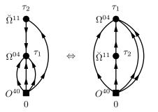
Figure 9: A BMBPT diagram drawn with some propagators going downwards (left) can be turned into an equivalent diagram with all its propagators going upwards (right) by moving the second vertex above the third one.
