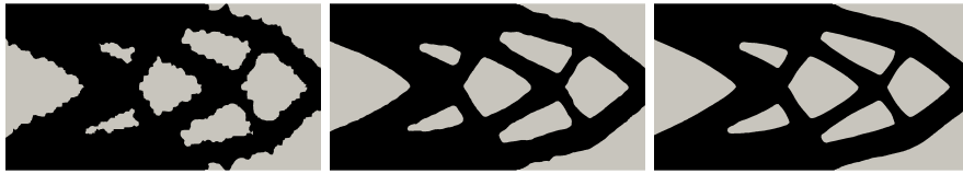
FIGURE 12. The Gauss-Newton algorithm with late start for the compliance of the cantilever, iterations 10,11,12 of the algorithm are shown
