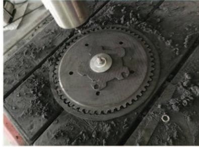
FIG. 4: Teeth cutting process on typical carbon/epoxy chainring
