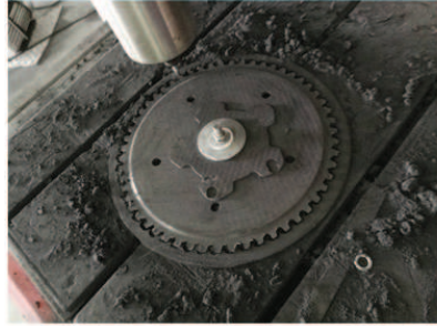
FIG. 4: Teeth cutting process on typical carbon/epoxy chainring
