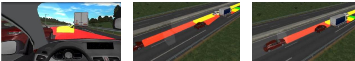
Figure 6. Simulation with COSMODRIVE of the decision making to manage a front collision risk (from a Lane Change versus a Braking)
