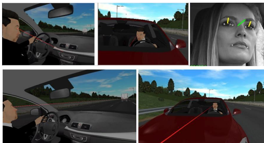
Figure 5. Replaying visual scanning with COSMODRIVE, from Eye tracking data collected among a real driver
