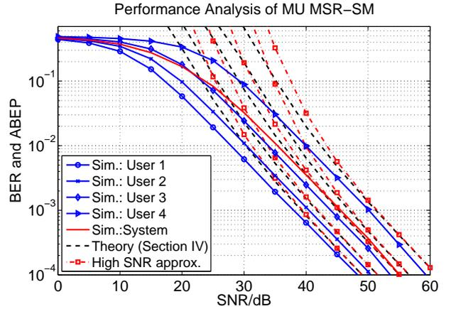
Fig. 3. Performance analysis of MU MSR-SM ( $N_s = 2$ ) for four users, when ZF with P-CSIT is employed: simulation results vs. the bounds in Section IV. The high SNR approximation of the ABEP is calculated using the PEP given in (32). Setup:  $N_t = 16$ ,  $N_r = 4$ ,  $\xi_i$ ,  $i = 1, \dots, N_u$ , takes the values 1, 0.75, 0.5, and 0.25 for the user 1, 2, 3, and 4, respectively.
