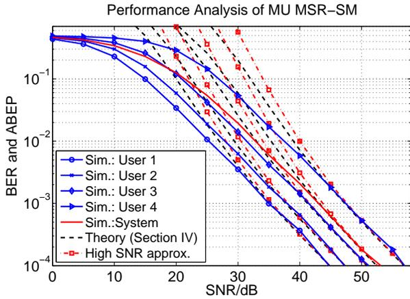
Fig. 2. Performance analysis of MU R-SM ( $N_s = 1$ ) for four users, when ZF with P-CSIT is employed: simulation results vs. the bounds in Section IV. The high SNR approximation of the ABEP is calculated using the PEP given in (32). Setup:  $N_t = 16$ ,  $N_r = 4$ ,  $\xi_i$ ,  $i = 1, \dots, N_u$ , takes the values 1, 0.75, 0.5, and 0.25 for the user 1, 2, 3, and 4, respectively.
