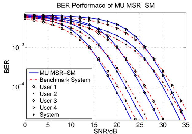
(b) The spectral efficiency is 8 bpcu, with  $N_s = 3$ .Fig. 6. BER performance of MU MSR-SM versus benchmark system (conventional MIMO broadcast channel with SMX). Setup:  $N_t = 20$ ,  $N_r = 4$ ,  $N_u = 4$ .
