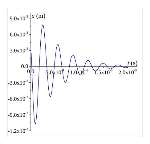
Figure 1: The time evolution of the displacement at the middle of the bar.
