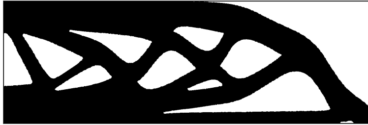
(C) Optimized shape with minimum thickness constraint ( d_{\min} = 0.2 ).
