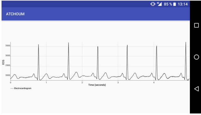
Fig. 4. Example of a 5 second period of ECG acquired by the sensor device and plotted on the smartphone's display.
