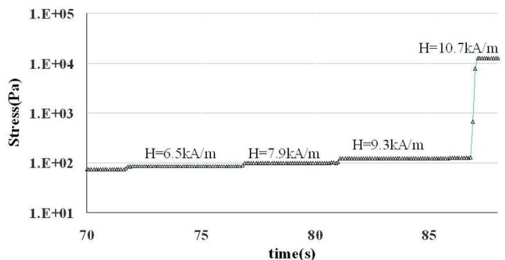
FIG.4 Increase of field step by step at a constant shear rate of  $10 \text{ s}^{-1}$
