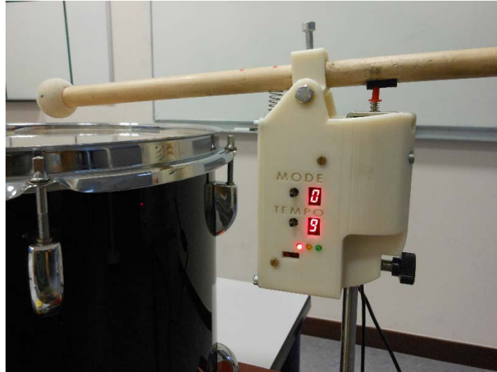
Figure 14. Final version of the MEM produced using professional FDM technology (year 2015)
