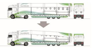
Fig. 4 Load Optimisation Combination with Double Floor Loading System and Aerodynamic Measures (adjustable roof, boat tail, side skirts)
