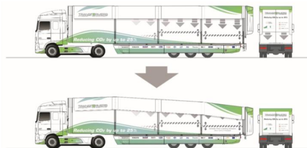
Fig. 4 Load Optimisation Combination with Double Floor Loading System and Aerodynamic Measures (adjustable roof, boat tail, side skirts)
