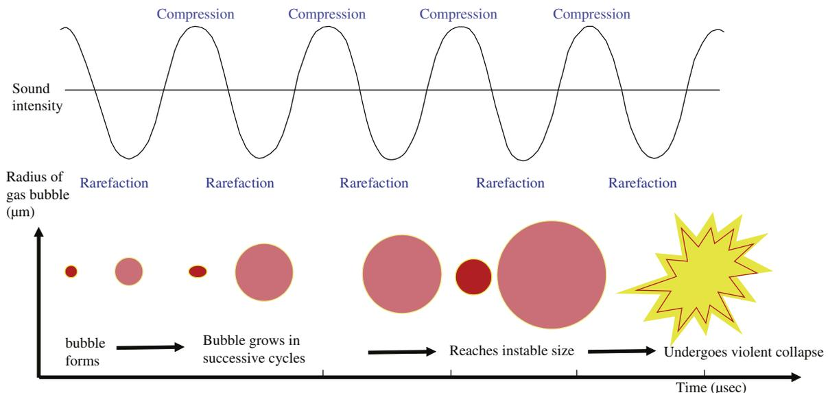
**Fig. 2 – Formation and collapse press of a cavity.**
