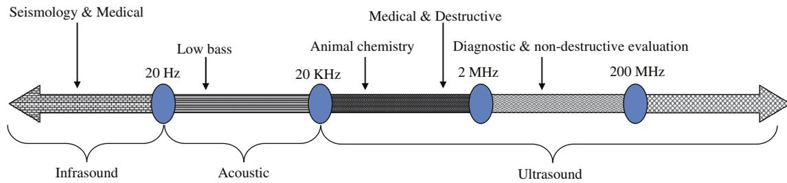
**Fig. 1 – Diagram of sonication range (Pilli et al., 2011).**
