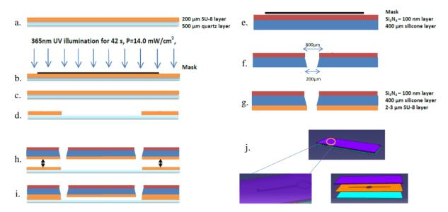
**Fig. 4**: Fluidic cell manufacturing process flow. a) SU-8 layer deposition on quartz layer. b) UV mask illumination c) Thermal treatment. d) SU-8 developer, rinsing. e) KOH etching. f-g) Conical configuration of inlet and output channels. h) Bonding parts g. and d. by thermal treatment. i) longitudinal cross section. j) 3D structure of the fluidic cell
