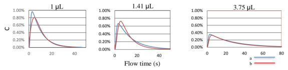
Fig. 3: Residence time distribution curves as area-weighted averaged concentrations at the outlet as a function of flow time
