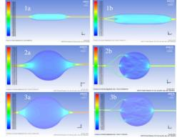
Fig. 2: Flow field velocity distribution in detection chamber: 1.  $1\mu L$  detection volume, **a**. one inlet channel, **b**. two inlet channels; 2.  $1.41~\mu L$  detection volume, **a**. one inlet channel, **b**. three inlet channels; 3.  $3.75\mu L$  detection channel. **a**. one inlet channel. **b**. three inlet channels
