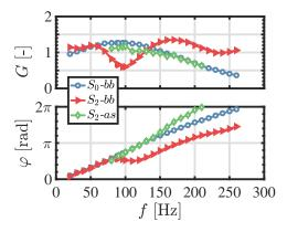
Fig. 2. Gain G and phase lag  $\varphi$  of the FTF for the three configurations investigated at the forcing level  $u'/\overline{u} = 0.30$  RMS.
