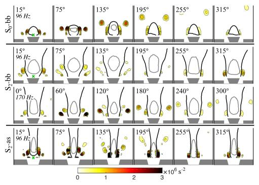
Fig. 5. Q criterion contour obtained from PIV measurements in cold flow conditions, for a forcing level  $u'/\overline{u} = 0.30$  RMS. Isolines of axial velocity are superimposed. Black contour:  $u_z = 0$  m/s. Gray contour:  $u_z = -2.5$  m/s. The position where the axial velocity  $u_z$  for the analysis of Fig. 4 is measured, is shown as a green cross at the phase 15°.
