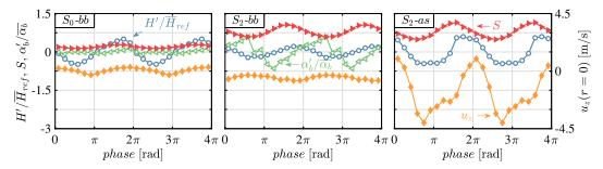
Fig. 4. Evolutions of the swirl number S and axial velocity  $u_z(r = 0)$  at the burner outlet with respect to the phase of the hot-wire signal. The relative flame height  $H'/\overline{H}_{ref}$  and flame base angle  $\alpha'_b/\overline{\alpha_b}$  oscillations are also plotted. Two oscillation cycles are represented for better readability.
