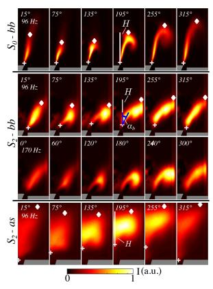
Fig. 3. OH\* intensity phase averaged images at a forcing level  $u'/\overline{u} = 0.30$  RMS. + : flame root position.  $\diamond$  : flame tip position.
