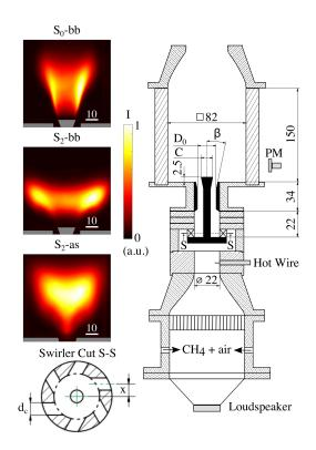
Fig. 1. Experimental setup.  $S_0$ -bb : Non-swirling flame anchored by a bluff-body,  $D_0 = 22$  mm, C = 14 mm.  $S_2 - bb$  : Flame stabilized by swirl S = 0.8 and the bluff-body,  $D_0 = 22$  mm, C = 14 mm.  $S_2$ -as : Swirling flame S = 0.75 stabilized aerodynamically,  $D_0 = 12$  mm,  $\beta = 15^\circ$ . The main dimensions are indicated in millimeters.
