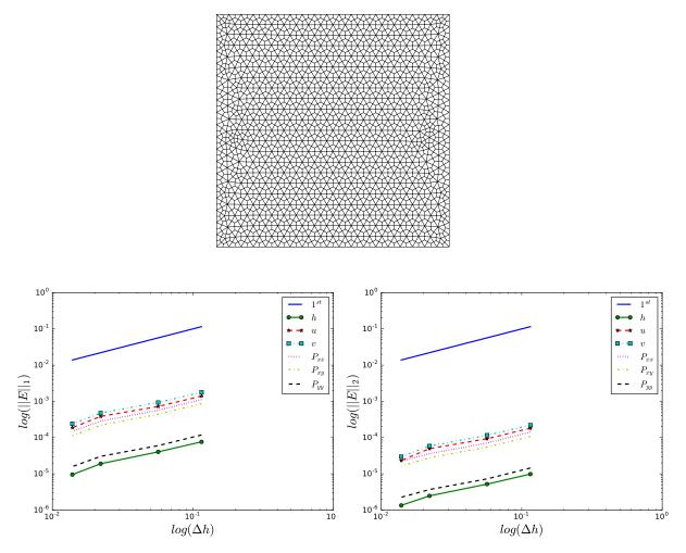
FIGURE 4. Unstructured quadrangular mesh :  $L_1$  and  $L_2$ -norm of the errors (E) plotted versus mesh size ( $\Delta h$ ) plotted on log-log scale at t = 10 s.
