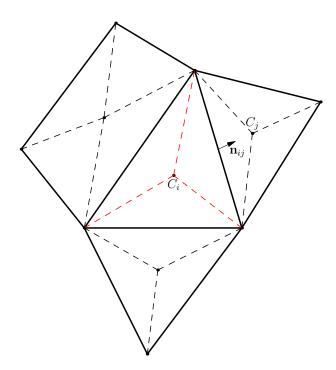
FIGURE 1. Sketch showing sub-cells formed in a cell  $C_i$ . Each sub-cell in the cell  $C_i$  shares an edge with cells  $C_j$  (cells surrounding a cell  $C_i$ ). The normal vector  $n_{ij}$  to the edge directs from the cell  $C_i$  to  $C_j$
