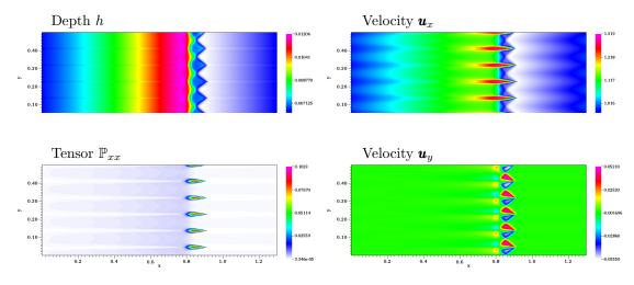
FIGURE 12. 2D roll waves : Top view of 2D roll waves with stable transverse structures at the time t = 57.8 s on structured quadrangular grid with  $1000 \times 400$  points and CFL = 0.4.
