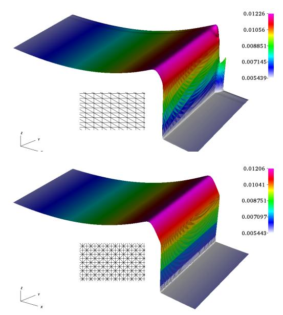
FIGURE 15. 2D roll waves : The depth (h) profile at time t = 40 s obtained on structured triangular grids with 206562 cells and CFL = 0.4. Top and bottom frames show results obtained on the grid with rectangles split in same and alternate orientation, respectively.
