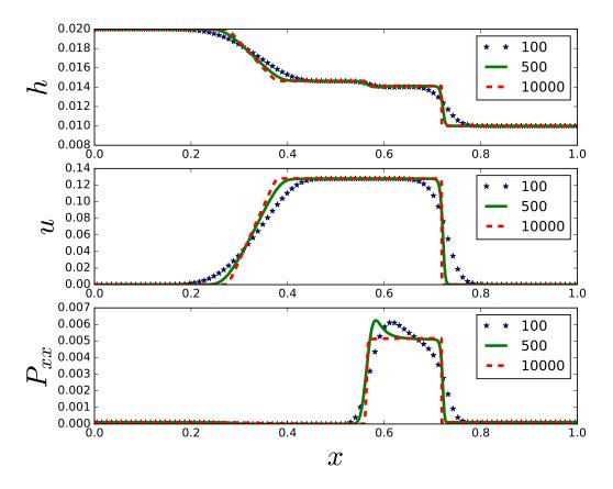
FIGURE 7. Numerical solution of 1D dam-break test showing h, u and  $\mathbb{P}_{xx}$  on the different grids with 100, 500 and 10000 grid cells. The CFL is specified as 0.8.
