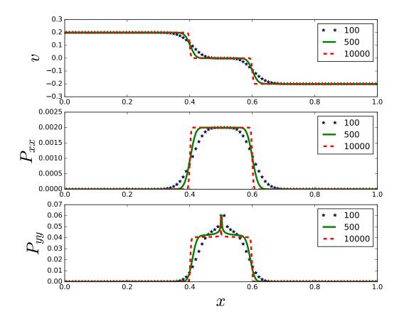
FIGURE 6. Numerical solution of 1D shear test showing v,  $\mathbb{P}_{xx}$  and  $\mathbb{P}_{yy}$  on the different grids with 100, 500 and 10000 grid cells. The CFL is specified as 0.5.
