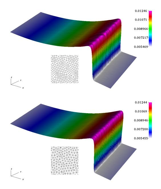
FIGURE 16. 2D roll waves : The depth (h) profile at time t = 40 s obtained with CFL = 0.4 on the unstructured quadrangular grid with 173251 cells (top) and on the unstructured triangular grid with 172898 cells (bottom).
