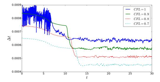
FIGURE 14. 2D roll waves : The curves of time-steps  $\Delta t$  plotted versus time t for the simulations of 2D roll waves on structured quadrangular grid with  $1000 \times 400$  points. Sharp decrease in each curve denote the onset of transverse waves.
