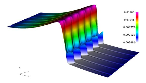
FIGURE 11. 2D roll waves : The depth (h) profile showing stable transverse structures at the time t = 57.8 s on structured quadrangular grid with  $1000 \times 400$  points and CFL = 0.4.
