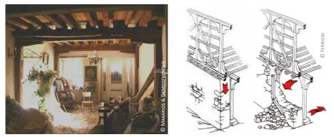
Greece, Lefkada Island: 1) inside timber frame; 2) behaviour of the double load-bearing system a) in ordinary situation and b) in case of an earthquake
