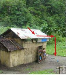
Philippines: rainwater is redirected away from the building thanks to a bamboo gutter
