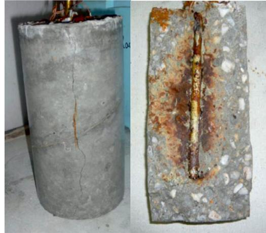
Fig. 4. Cracks on the material and corrosion of the stainless steel bar (28 day-treatment at 5 A/m<sup>2</sup>).
