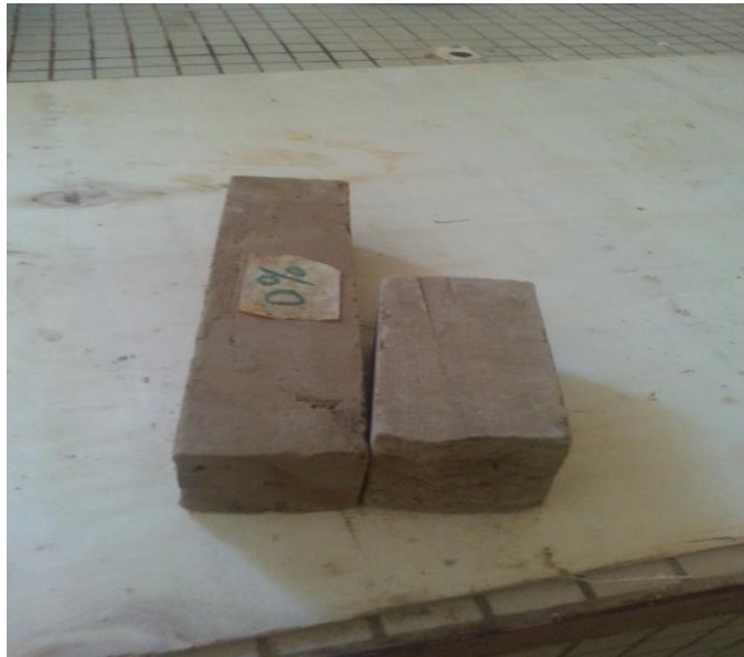
Fig.3: The samples before and after the flexural strength test
