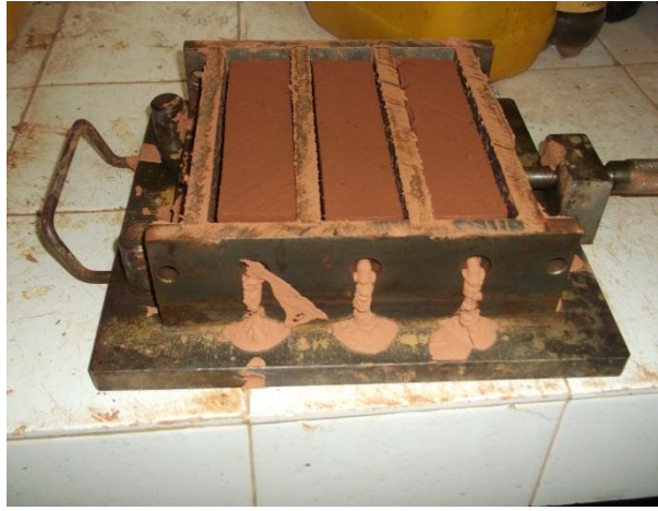
Fig.2: Picture of the paste within the prismatic moulds
