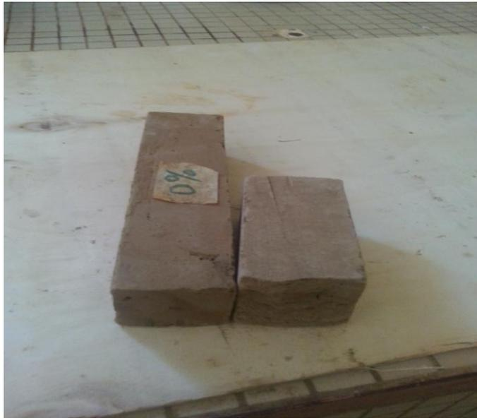
Fig.3: The samples before and after the flexural strength test
