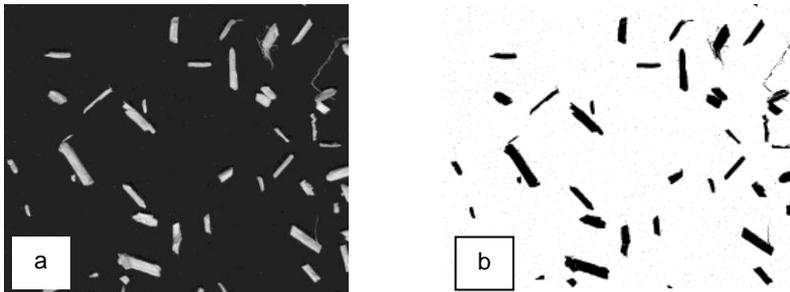
198 **Fig.3** Particle image processing of straw: (a) Scan in shades of grey, (b) Image processing
