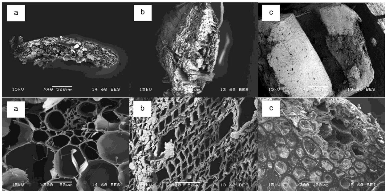
350 **Fig.7** SEM images of: (a) straw, (b) hemp shiv and (c) corn cob at low (first line) and high
