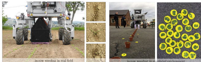
Fig. 6: Left: an in-row mechanical weeding and spraying test is conducted in the real-world field in Ancona, IT. The weeds after spraying can be seen in the picture, and the mechanical treatment results are not visible on the ground. Right: the performance of in-row mechanical weeding is presented in a simulated test environment in Bonn, GE. The faked targets made of leaves attached to modeling clay is utilized to visualize the execution results.
