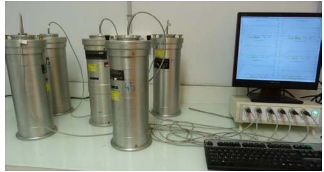
Fig. 3. Semi-adiabatic calorimeters for hydration test.
