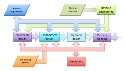
Fig. 1 Generic structure of a PDP and its associated flows of information and/or digital models [22]
