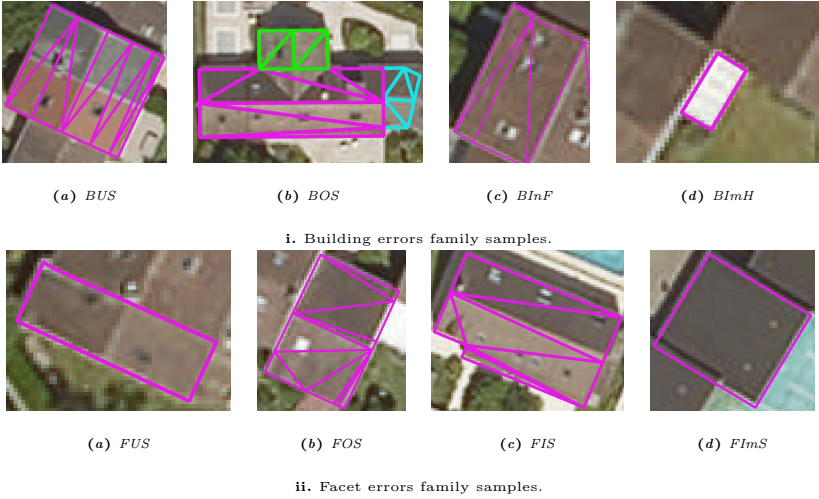
Fig. 3: Illustration of various errors of our taxonomy. One can see that geometric, spectral and height information are required for an accurate detection of all kinds of errors.
