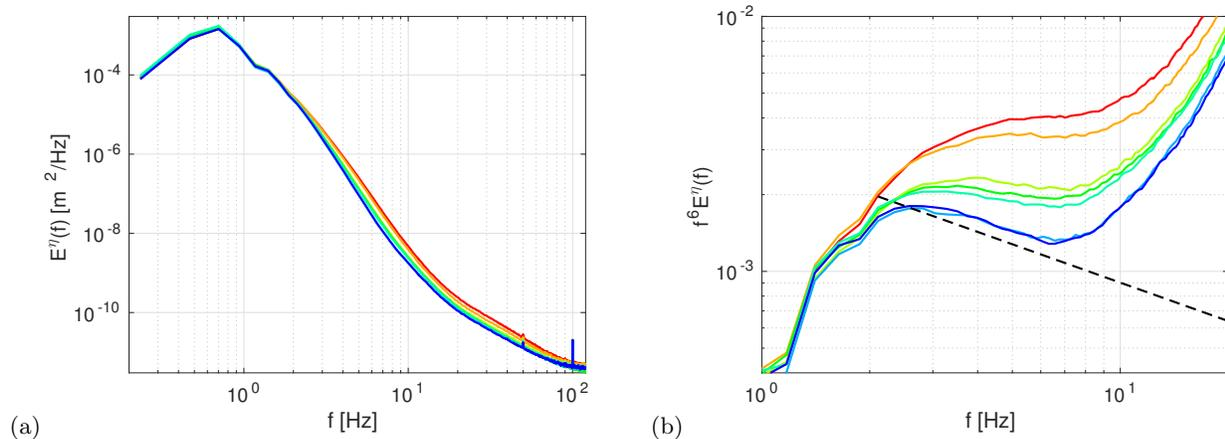
Figure 5. Evolution of the wave spectrum versus time for weakest forcing. Each curve corresponds to an average over the 10 probes and a time average over one hour of continuous recording (7 successive records from red to blue). (a) Wave elevation spectrum  $E^\eta(f)$ . (b) compensated spectrum  $f^6 E^\eta(f)$  in the low frequency range. The dashed line is  $\propto f^{-0.5}$ .
