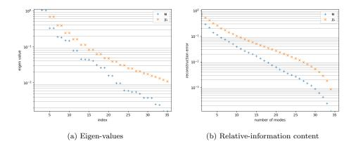
Figure 5: Eigen-values (left) of the temporal correlation matrix (A.8) and reconstruction error (32) associated with the velocity field u (+) and the rigid body characteristic function  $\chi_{s}$  (×).
