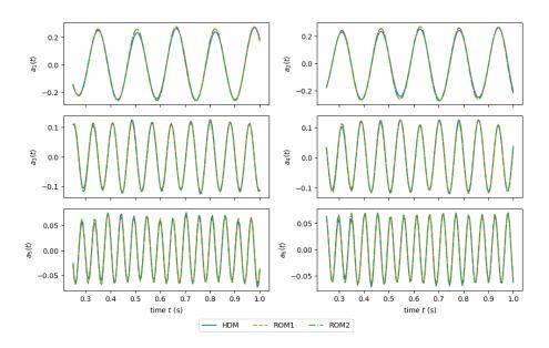
Figure C.12: Temporal evolution of the coefficients for the fluctuating part of the velocity in the steady case (see 5.2.1).
