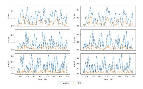
Figure 11: Error on the coefficients for the fluctuating part of the velocity in the the interpolation case (see section 5.3). The definition of the error is in equation 34).
