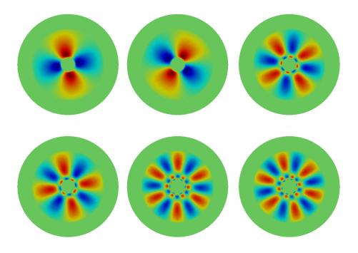
Figure 4: First modes for characteristic function  $(\phi_i^{\chi})_{1 \le i \le 6}$  for both the steady and the transient cases (from left to right and top to bottom).
