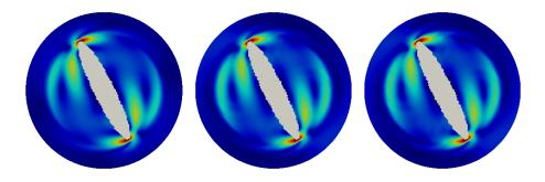
Figure 6: Magnitude of the fluctuating velocity  $\boldsymbol{u}(\boldsymbol{x},t) - \overline{\boldsymbol{u}}(\boldsymbol{x})$ . Left: HDM. Middle: ROM1. Right: ROM2.
