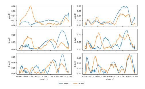
Figure 10: Error on the coefficients for the fluctuating part of the velocity in the transient case (see section 5.2.2). The definition of the error is in equation 34).
