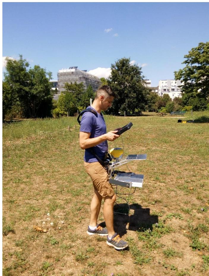
UHF RFID detection device
