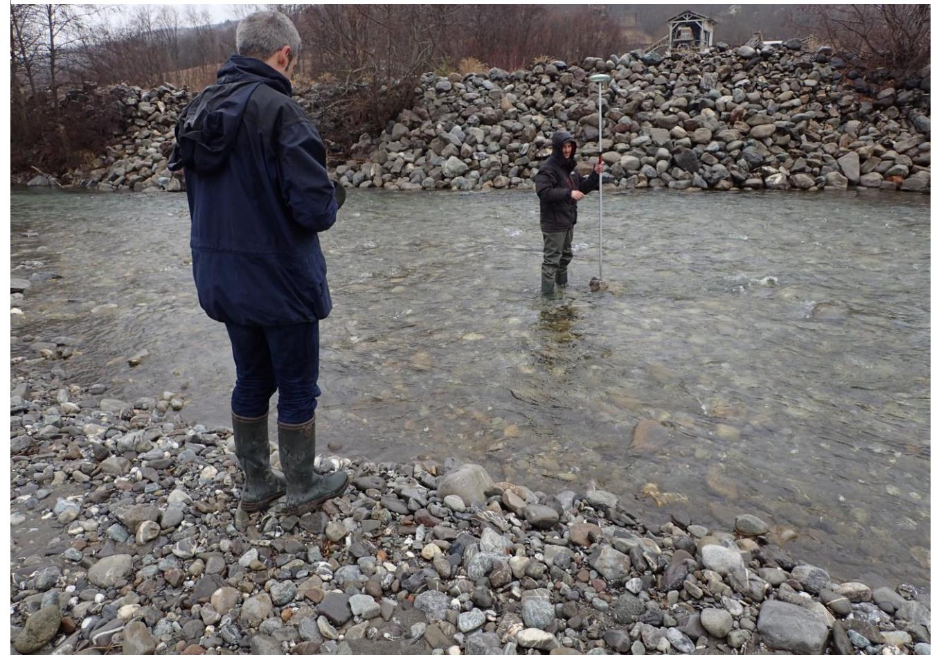
Cross section with RTK GPS
