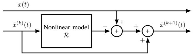
Fig. 3.  $k$ -th stage of the signal-optimized signal predistortion [5]–[8].
