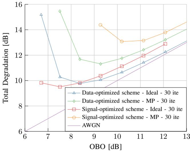
Fig. 7. Total degradation with ACI for a target BER of  $10^{-4}$  for the data-optimized and the signal-optimized signal predistortion scheme with perfect knowledge of the channel (Ideal) or with identification (MP).
