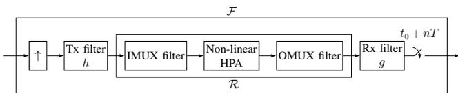
Fig. 2. Relation between the data-based and the signal-based model.
