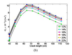
Figure 7: Evolution of GI versus moisture content for different temperature variation (a); Evolution of GII versus moisture content for different temperature variation (b).
