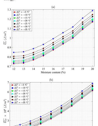
**Figure 8:** Evolution of  $G_I$  versus moisture content for different temperature variation (a); Evolution of  $G_{II}$  versus moisture content for different temperature variation (b).
