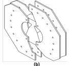
Figure 2: (a) MMCG wood specimen – (b) Modified Arcan fixture
