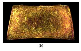
Figure 9: 3D volume visualisation of Padouk sample under moisture variation (a); 2D cross sectional visualisation of moisture effect on internal crack growth (b).
