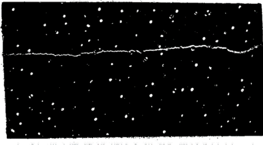
Figure 5: Crack properties extraction using image analysis.
