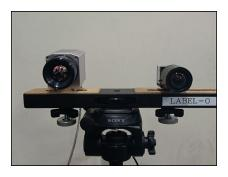
Figure 12: **Camera rig.** Left: thermal-infrared camera. Right: RGB camera.
