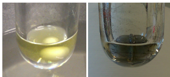
Figure 3: Photos of the [IrCl(COD)MesImPr] catalytic solution before (a) and after (b) catalytic reduction of Terpinen-4-ol at 80 °C with 0.1mol% of catalyst.
