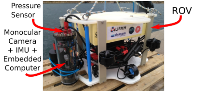
Fig. 1. The Remotely Operated Vehicle (ROV) and acquisition system used to record the dataset.
