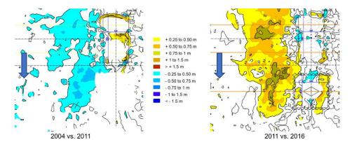
Fig. 3. Results of comparison between 3 bathymetry campaigns (2004, 2011 and 2016) near the pier 4 of the A71 highway viaduct over the Loire river. (Blue arrow: flow direction)
