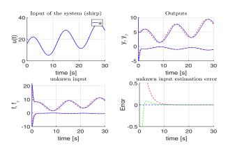
Fig. 1. Input (u)-output (y) and its delayed value  $(y_{\tau})$  -unknown input with delay  $(F-F_{\tau})$  and the error.
