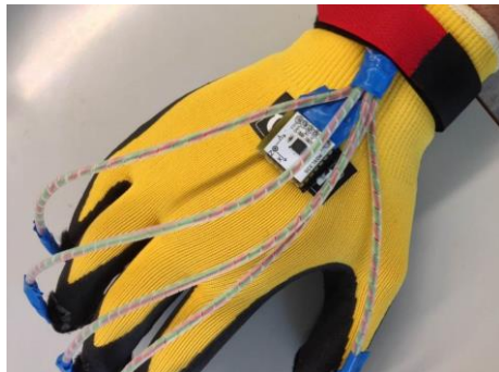
Figure 1: Sensor glove system with force sensors and acceleration sensor.
