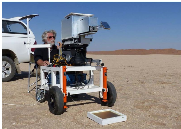
Figure 3. Instrumentation setting used for in situ measurements of emissivity soundings.
