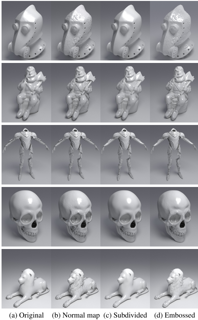
Figure 11: Embossing results. We subdivide (c) the input model (a), and emboss the normal map (c) onto the subdivided model (d). When shading normals are not aligned with geometric normals, physically-based renderers can produce artifacts such as black regions (b) if not handled with particular care.
