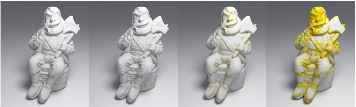
Figure 7: Influence of \lambda on denoising results. First row: Original and noisy models. Second row: denoising with \lambda = 0.05 (left) and \lambda = 0.01 (right). Decreasing \lambda produces longer features, and more discontinuities.
