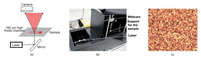
Fig. 1 (a) Schematic and (b) image of the transmission setup, where the sample is placed between the laser and the camera. (c) Typical speckle image recorded on a whole-blood sample.
