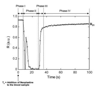
**Fig. 2** Addition of Neoplastine to the blood sample at  $T_0$  triggers the coagulation dynamics. After a first phase corresponding to the homogenization of the solution in tube (phase I), the sample is introduced in the chamber by capillary forces, leading to blood cells motion (phase II). Upon coagulation the cells motion suddenly slows down (phase III), before their complete immobilization in the clot (phase IV).
