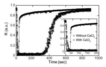
**Fig. 4** In the absence of calcium chloride, coagulation cannot take place. Variation of the correlation coefficient versus time, with (open circles) and without calcium chloride (crosses) for the same blood sample. The inset shows a close-up on the first 200 s.
