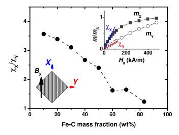
FIG. 3. Dependence of the pillars' magnetic anisotropy as a function of the Fe-C doping fraction. The inset shows how  $\chi_X$  and  $\chi_Y$  are determined from the reduced magnetization curves of a 30wt% composite pillar.
