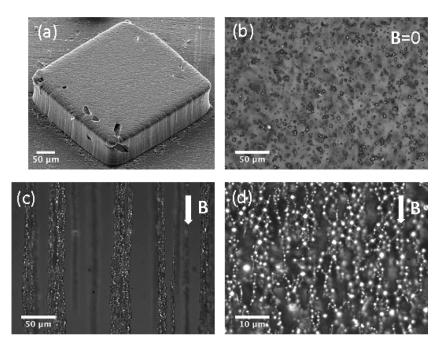
FIG. 1. (a) SEM image of a composite microstructure (500 µm diagonal diamond shape). Optical images of 10w% I-PDMS composites of S0 (b) and S130 (c) series, and 83w% I-PDMS of S130 (d).
