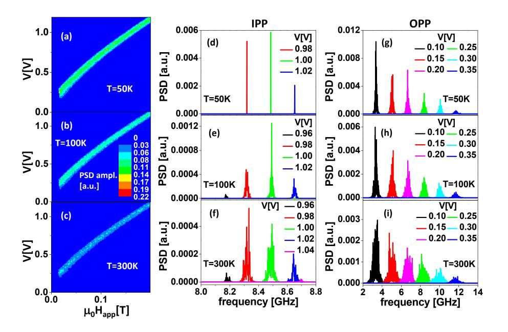
FIG. 5. Power spectral density (PSD) peak amplitude representation as a function of voltage and field at (a) T=50K, (b) T=100K, and (c) T=300K. PSD representation at constant field ( $\mu_0 H_{app}=0.3T$ ) and K<sub>2</sub>=0 (IPP mode) for different voltage values at (d) T=50K, (e) T=100K, and (f) T=300K. PSD representation at constant field ( $\mu_0 H_{app}=0.001T$ ) and K<sub>2</sub>=-120 kJ/m<sup>3</sup> (OPP mode) for different voltage values at (g) T=50K, (h) T=100K, and (i) T=300K.
