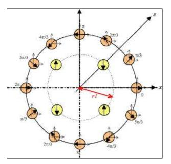
Figure 8: Direction of magnetization of the 8 shim magnets.
