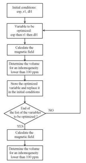
Figure 9: Flow chart of our configuration with 24 main magnets and 8 shim magnets.
