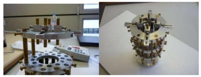
(a) Shim magnets that can move along three degrees of freedom.
