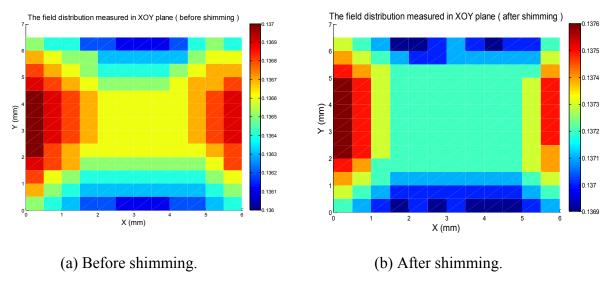
Figure 19: Magnetic field homogeneity at z = 0 in xOy plane.
