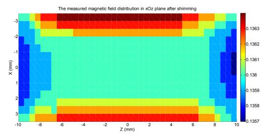
Figure 20: The magnetic field homogeneity in xOz plane after shimming.
