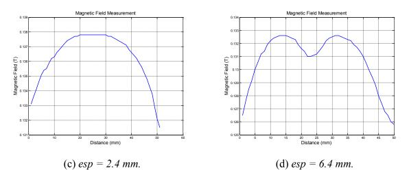
Figure 16: Magnetic field profiles in Oz direction for different esp values.
