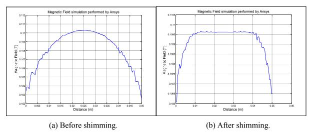
Figure 12: Magnetic field profiles at the center of our Halbach arrangement of magnets.
