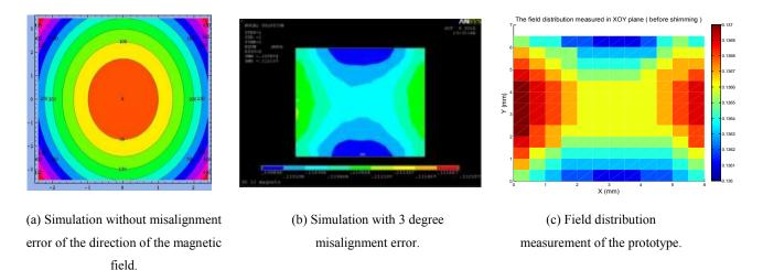
Figure 23: The magnetic field distribution in xOz plane, for ideal case and with error of misalignment of the direction of the magnetic field.
