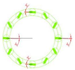
Figure 22: Misalignment of the magnetic direction for four magnets.
