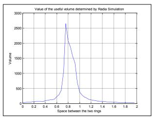
Figure 6: Volume (mm<sup>3</sup>) for a variation of  $\frac{\Delta B_0}{B_0}$  lower than 100 ppm is a function of the gap
