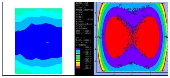
(a) Before shimming. (b) After shimming. Figure 10: Magnetic field homogeneity in the xOy plane and z = 0.
