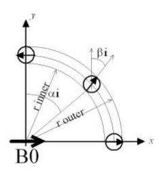
Figure 1: Geometric parameters of Halbach structure.
