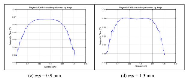
Figure 5: The field profile for different values of the gap *esp* between the two rings.
