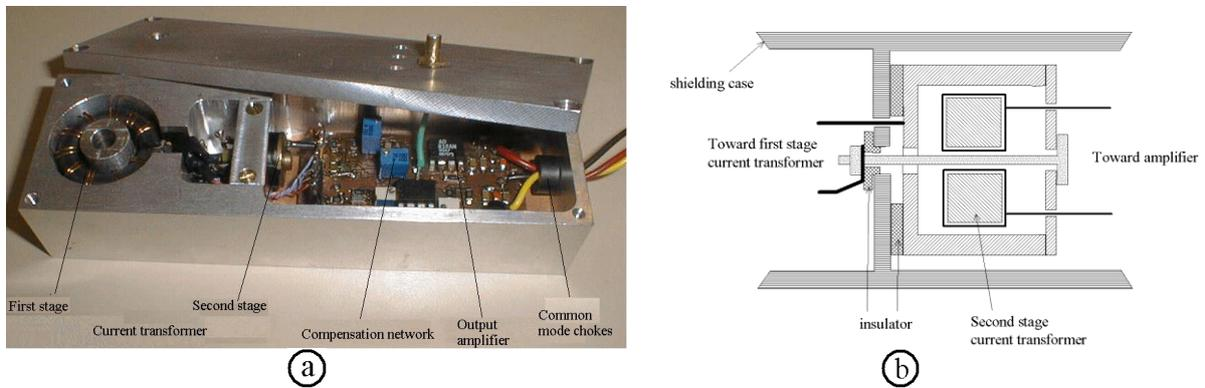
**Fig. 12: (a) Picture of the ACT<sup>2</sup>. (b) Detail of the ACT<sup>2</sup> second stage.**
