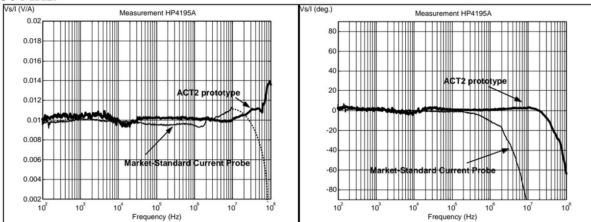
**Fig. 10:** Comparison between the ACT<sup>2</sup> and a market-standard current probe.
